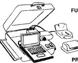
FUNCTION: Provides direct access into CI/HUMINT collateral LAN; uses INMARSAT, TROJAN SPIRIT, SINCGARS, MSE, DSN & phone lines; 2-way data comm; secure FAX; future: GPS, cellular comm, power mgt
