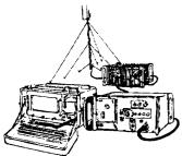
FUNCTION: Communications terminal; GUARDRAIL downlink on TRIXS network; RRS on board RC-12 & U2-R, RRTS; includes OT, RBP, RRT, LOS adaptive array antenna, SDS, embedded COMSEC
